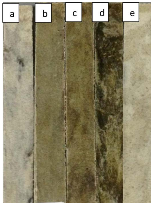
Figure 4. Flexural samples before weathering: (a) rHDPE, (b) 10 wt % PCB, (c) 30 wt % PCB, (d) 40 wt % PCB, and (e) 6 phr MAPE: Addition of nonmetallic PCB into rHDPE matrix turned the composite to darker color (b–d), while addition of MAPE made the color of composite lighter (e). [Color figure can be viewed in the online issue, which is available at wileyonlinelibrary.com .]
