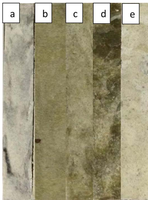
Figure 5. Flexural samples after 2000 h of accelerated weathering: (a) rHDPE, (b) 10 wt % PCB, (c) 30 wt % PCB, (d) 40 wt % PCB, and (e) 6 phr MAPE: All the composites tend to become lighter in color upon exposure to accelerated weathering. [Color figure can be viewed in the online issue, which is available at wileyonlinelibrary.com .]
